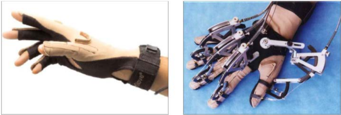
Figure 7: Left: A 15 DOF Tracking Glove. Right: A mechanical exoskeleton for force feedback (images from CyberGlove Systems)
